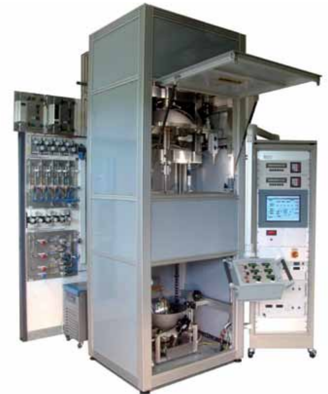
Fig.4 The so called ‘mirror ovens’ that are used to produce large single crystal of the complicated oxides and other materials that form the environments where the “quantum matter” electron systems are found.
