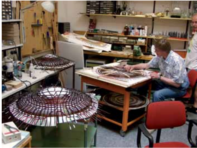
Experimental gradient coil, according to which the magnetic field strength in the patient is varied locally (Philips Research).
