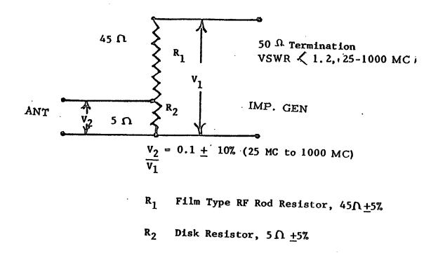
Fig. 4 - Injection Network Characteristics (25 to 1000 MC)
