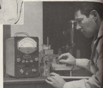
Measuring surface potentials of PN junction on germanium crystal specimens at IBM
