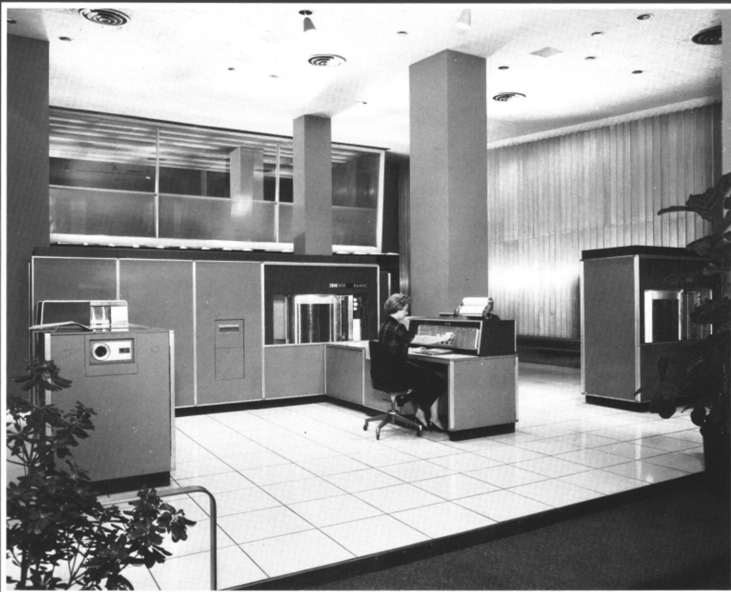
One of the press release photos for the 305 RAMAC System when it was first announced in 1956. Key component was the 350 disk file. The system also included a central processor, card reader and printer.
