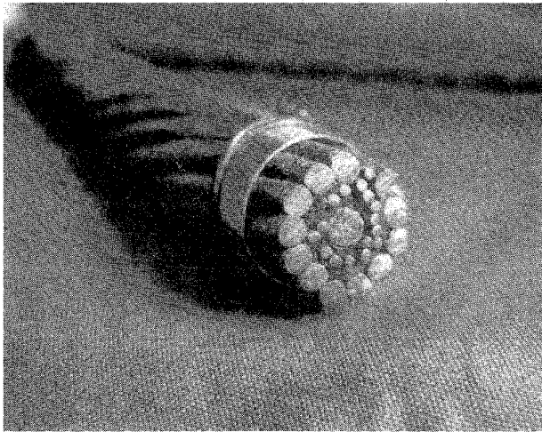
Figure 1. A deep-sea submarine telegraph cable, circa 1900, cut to show the cross-section (a cable in the collection of the French Cable Station Museum).
