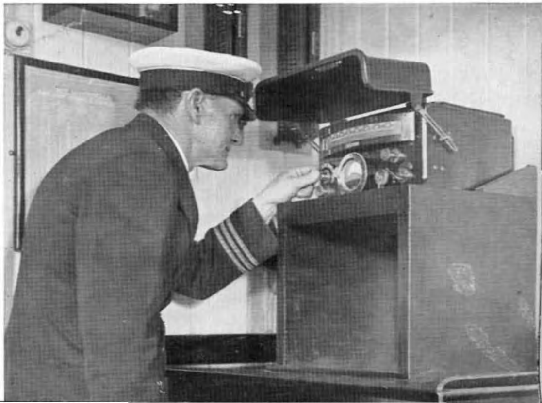
Depth Sounding Apparatus installed on Trans-Tasman Liner.
