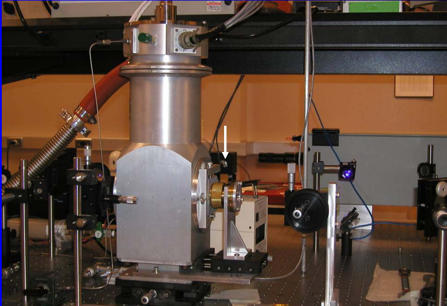
HPDC for in-situ synthesis, fast quenching and characterization
