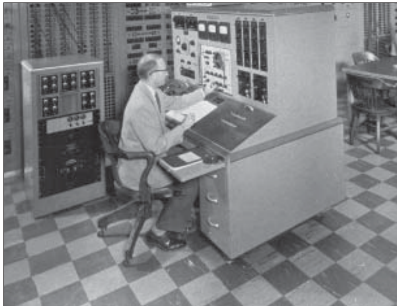
Figure 9. The Anacom analog computer was used to simulate complex electric power networks.
