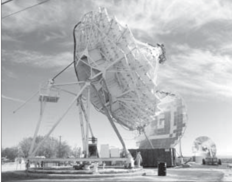
Figure 19. A solar power unit developed by the Jet Propulsion Laboratory to drive a Stirling engine, 1982.
