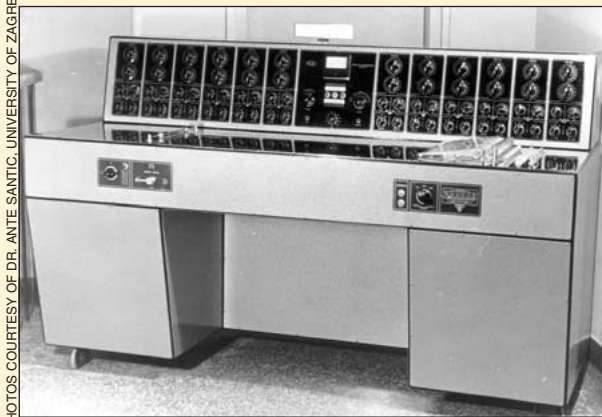
PHOTOS COURTESY OF DR. ANTE SANTIĆ, UNIVERSITY OF ZAGREB Front (above) and rear (below) views of a 12-channel electroencephalograph developed in Southeastern/Central Europe in 1960 at the Institute of Electrical Engineering in Zagreb, Croatia.
