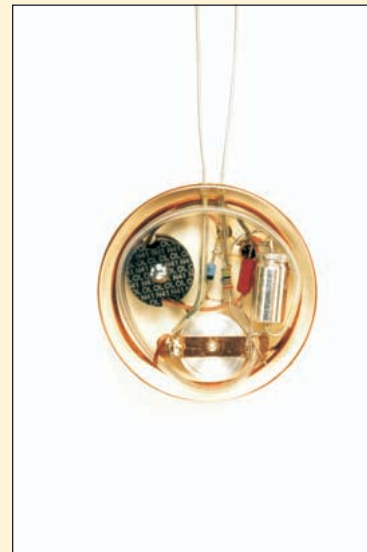
The first implantable pacemaker was developed through collaboration by cardiac surgeon Dr. Ake Senning and Dr. Rune Elmqvist in Sweden. Arne Larsson in 1958 was the first person to receive the device. This pacemaker used two transistors and was the size of a hockey puck.
