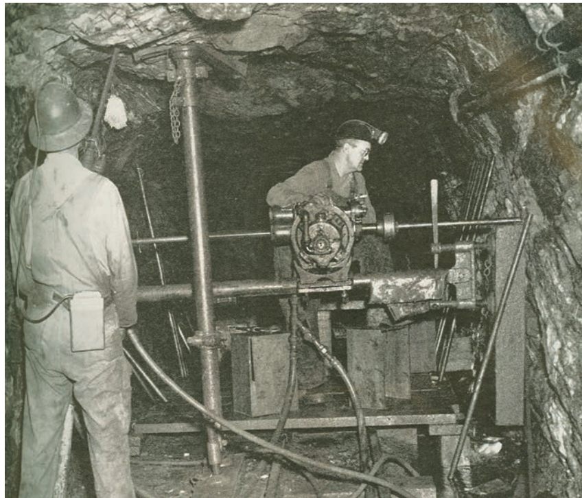
A diamond drill station in operation in 1957 at Homestake Mining's historic Homestake gold mine in Lead, SD.
