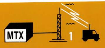
During conversation the base station sends a continuous supervisory signal which is returned by the mobile station. The signal-to-noise ratio of the returned signal is measured in the base station and found satisfactory.
