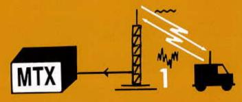
As the mobile station moves further away from the base station the signal-to-noise ratio deteriorates. When a critical value is passed the base station sends alarm to the MTX.
