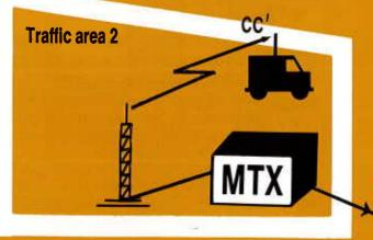
The mobile station now locks to the calling channel in traffic area 2. From the MTX an updating message is sent to the mobile station's home MTX about its new position.
