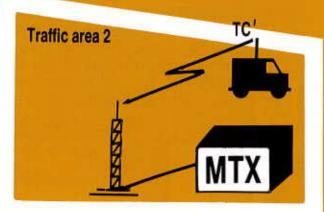
The mobile station finds a free traffic channel. A frame for updating of roaming is sent. The MTX returns an acknowledgment.
