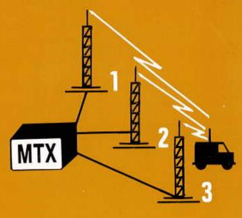
The MTX orders the actual and neighbouring base stations to measure the signal strength on the channel. The base stations return the results of the measurements to the MTX. In the example illustrated, base station 3 measures a considerably higher signal strength than base station 1.
