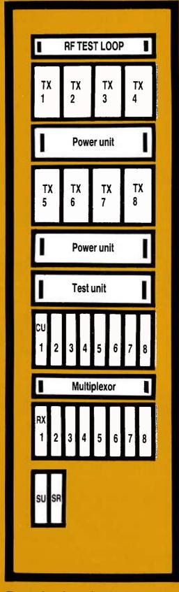
Example of mechanical structure of an 8-channel station. Apart from the radio racks shown, two additional racks containing transmitter combiners are needed.
