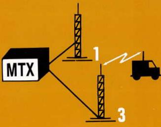
The MTX decides that the call must be switched to base station 3. The mobile station is ordered over to another traffic channel and at the same time base station 3 starts a handshaking procedure on the same channel (cf. call to mobile subscriber). Base station 1 is disconnected.
